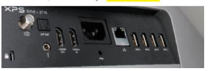
The HDMI and S/PDIF outputs on the XPS One are much more useful than the VGA input on the Asus.
